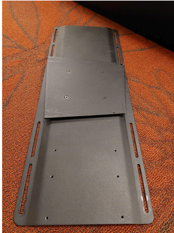
Image 13: Pressure plate where the television is secured
