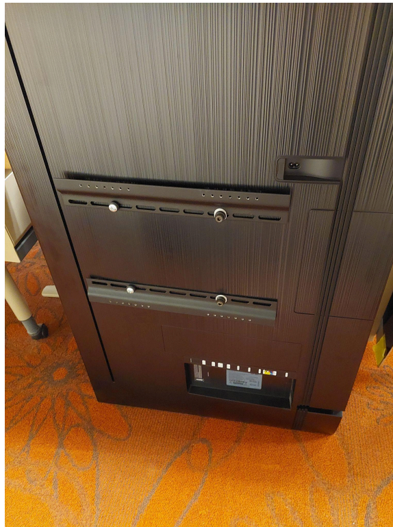
Image 18: Television back disconnected from frame and rotated to new orientation
